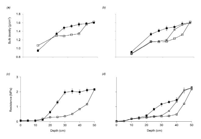
FIGURE 2. EFFECT OF DESTONING DEPTH ON SOIL BULK DENSITY AND PENETRATION RESISTANCE. BULK DENSITY: (*A*) EXPT 1; (*B*) EXPT 2. RESISTANCE: (*C*) EXPT 1; (*D*) EXPT 2. ■, SHALLOW; ■, NORMAL; □, DEEP. MEAN OF TWO N REGIMES IN EXPT 1 AND TWO AGGRESSIVENESS TREATMENTS IN EXPT 2.
